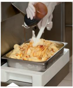
To better variegate gelato coming out, the extraction speed can be reduced and varied as desired, allowing the easy distribution of toppings. The shelf mat is designed to firmly hold trays and tubs in position while gelato is being worked on.
