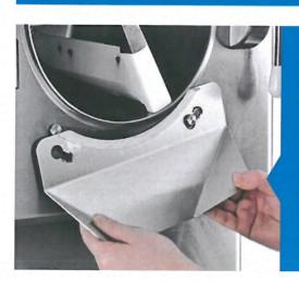
With the hot-cleaning of the cylinder and the removable gelato chute, cleaning is easier.
